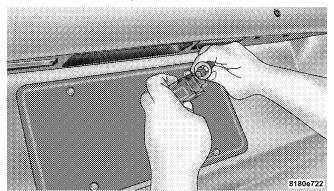
Removing Socket From Lamp
